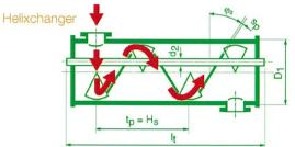
line of the exchanger. Successive baffles are arranged in such a way as to create continuous helical and near
